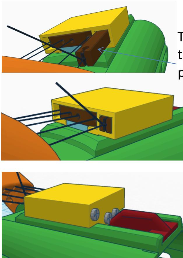
Cut a length of thread twice as long as the hand and tie it using a triple knot through the small hole at one end of the thumb tensioner pin. Pull the knot tight using two pairs of small long nose pliers. Cut the excess thread to about an inch long. Thread the long end of the thread through the remaining hole in the back of the palm and down to the end of the thumb tip as you did with the fingers. Don't tie it to the end of the thumb tip yet!
