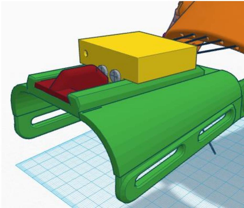
Insert and tighten two of the pan head sheet metal screws so that they attach the swivel pin. The screw heads should both be flush with the back of the gripper box but the swivel pin should still be as far forward in its slot as possible.
