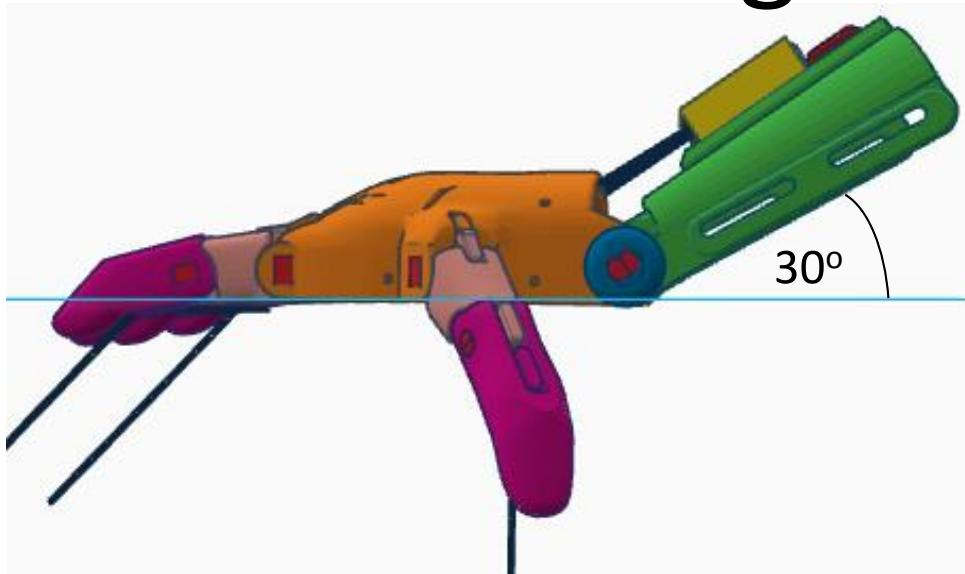
Raise the gauntlet so that it has an approximately 30° angle to the palm. Turn the hand upside down and place it at the edge of a table with the fingers overhanging.
