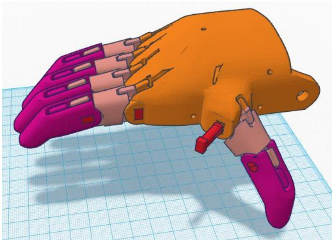
insert the thumb into its joint slot then push the thumb knuckle pin in fully. This can usually be done using just the pliers.
