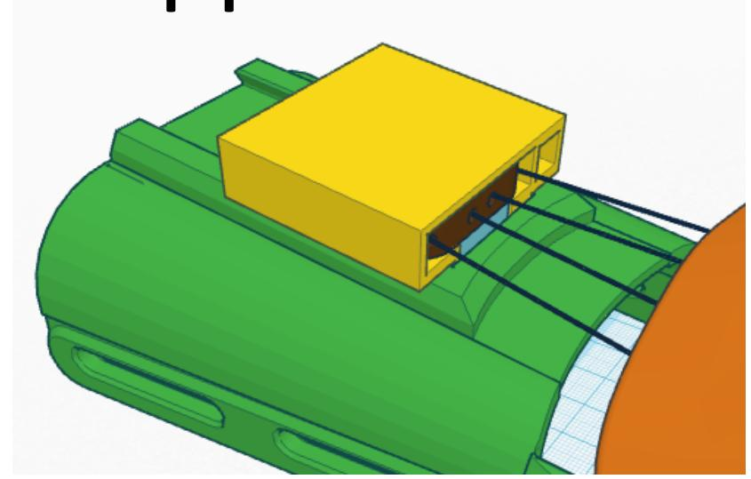
Insert the swivel pin under the whippletree in front of the gripper box. Then slide the gripper box forward as far as it can go. The whippletree will now be entirely enclosed within the gripper box.
