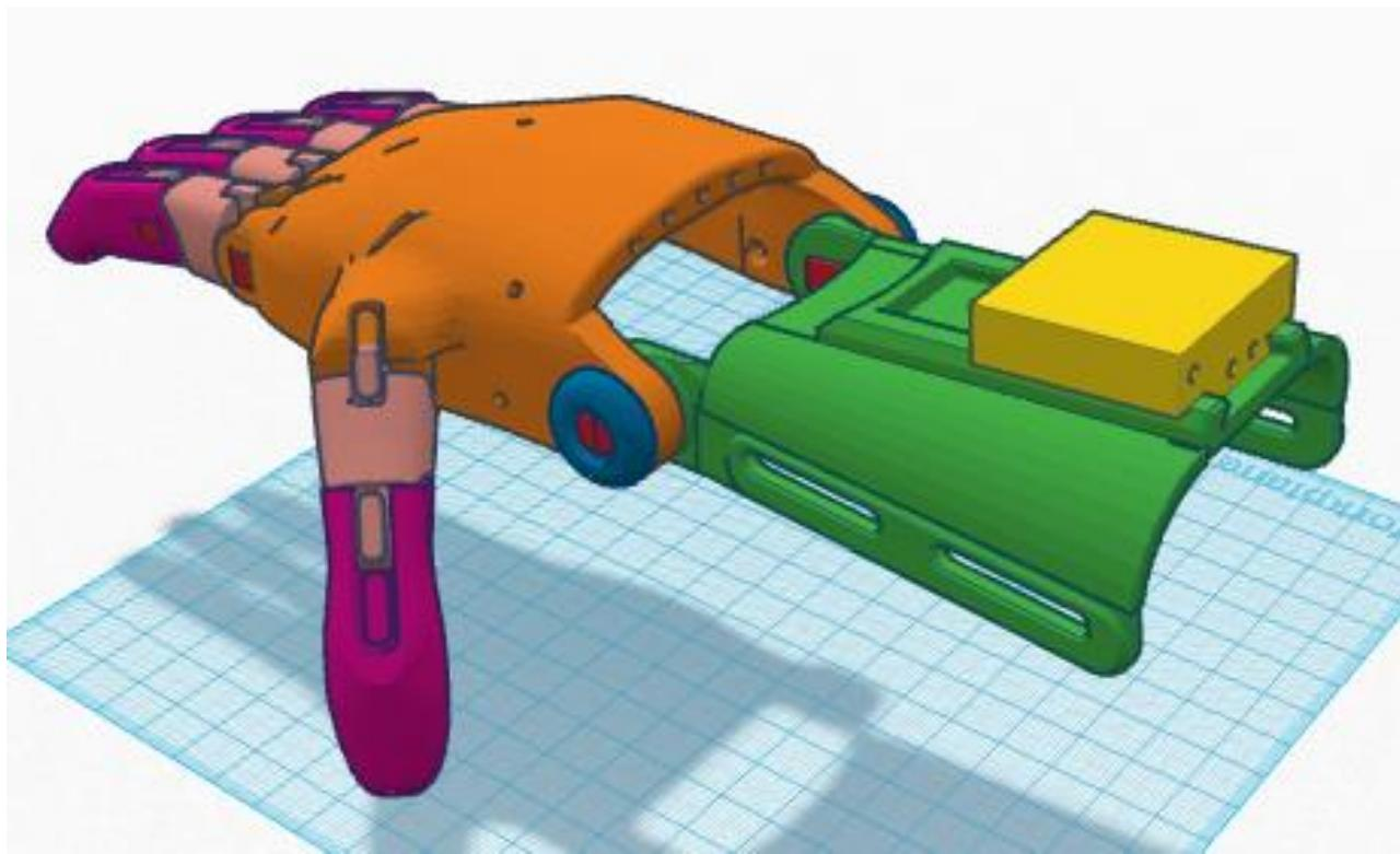
Push the gripper box into the dovetail slot on the back of the gauntlet but only push it far enough for the back of the gripper box to be fully in the slot. This is to allow the components to be fitted inside in a subsequent step.
