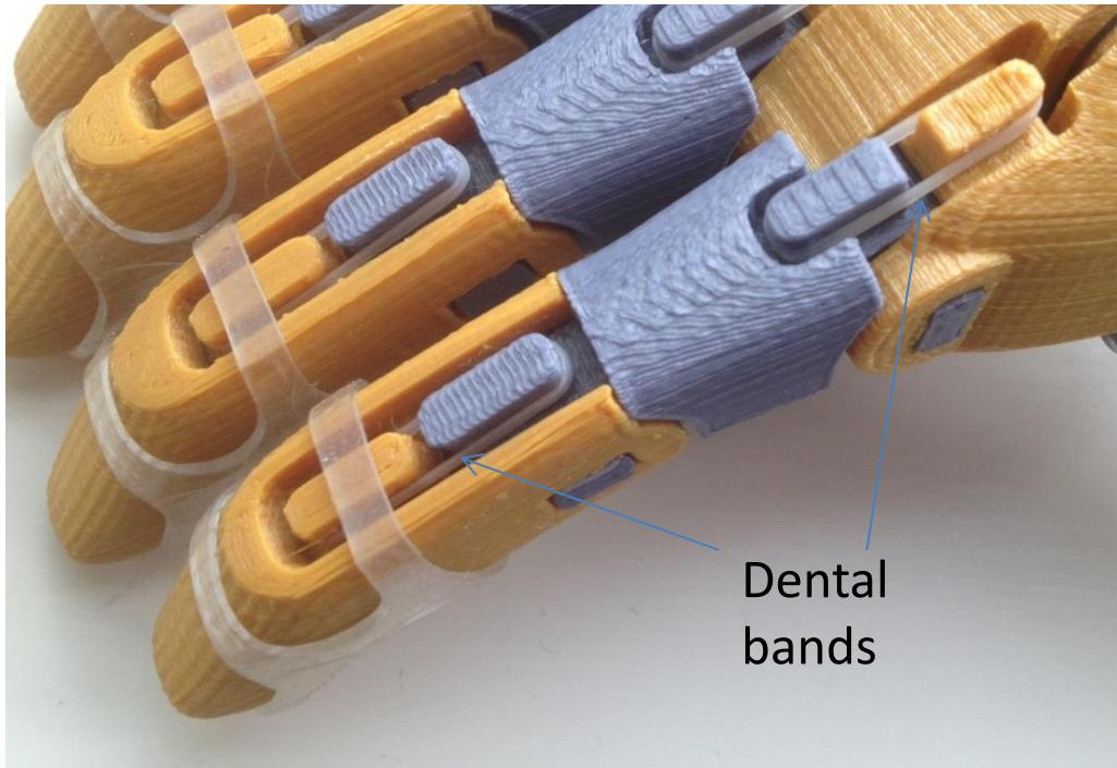
Using a thin pointed tool such as a toothpick attach dental bands to each of the the ten finger and thumb joints. The bands will pull the fingers and thumb into their straight unclenched position.
