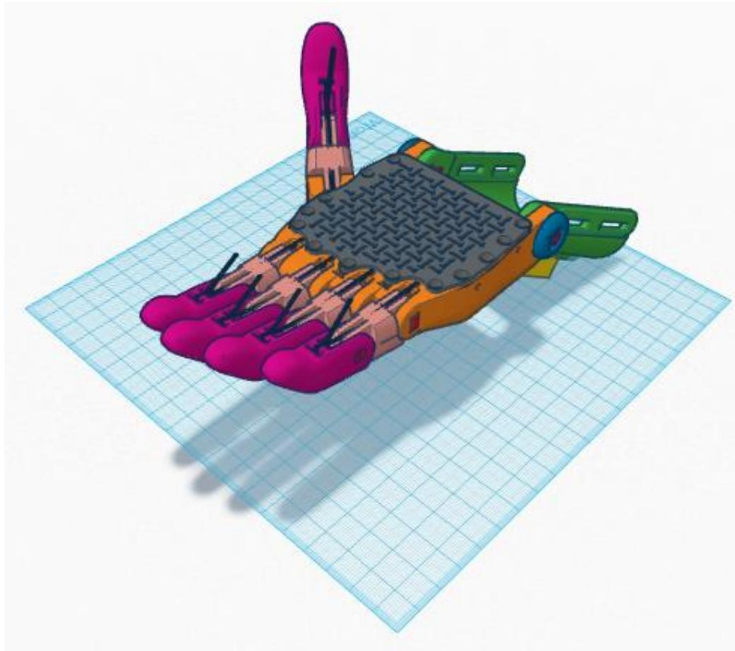
Screw the palm mesh to the palm using 13 countersunk wood screws.
