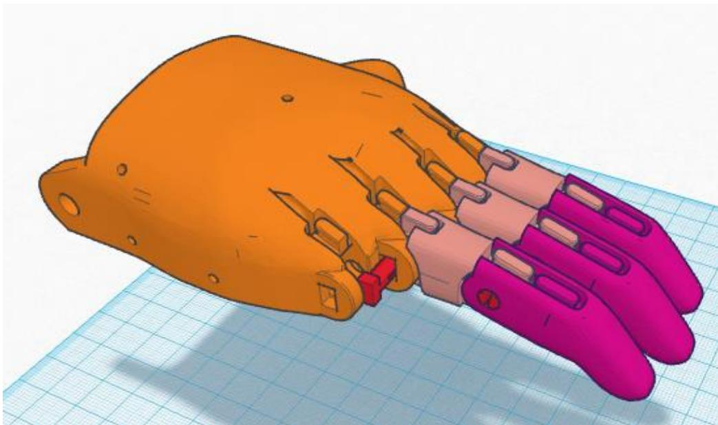
Before inserting one of the short knuckle pins ensure that its rectangular head will fit in the rectangular ring finger hole in the palm. If necessary file or sand the pin head to fit.
