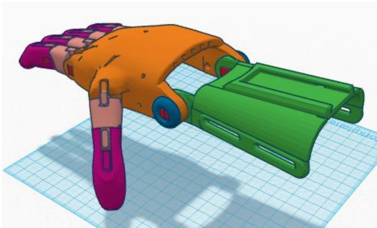
Snap the wrist pin caps onto the ends of the wrist pins. You may need to squeeze the cap onto the pin using the pliers on their wide jaw setting.
