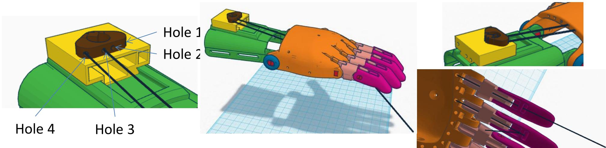
Place the whippetree on the back of the gripper box with the four holes facing the palm and the smoothest surface touching the gripper box. You'll need to hold it there while stringing the remaining fingers. Pass the thread from the ring finger through hole 3 on the whippetree and back out though hole 4. Now thread it into the fifth hole from the thumb side on the back of the palm and down through the pinkie fingertip as you did with the other fingers. Don't tie a knot at the end yet!
