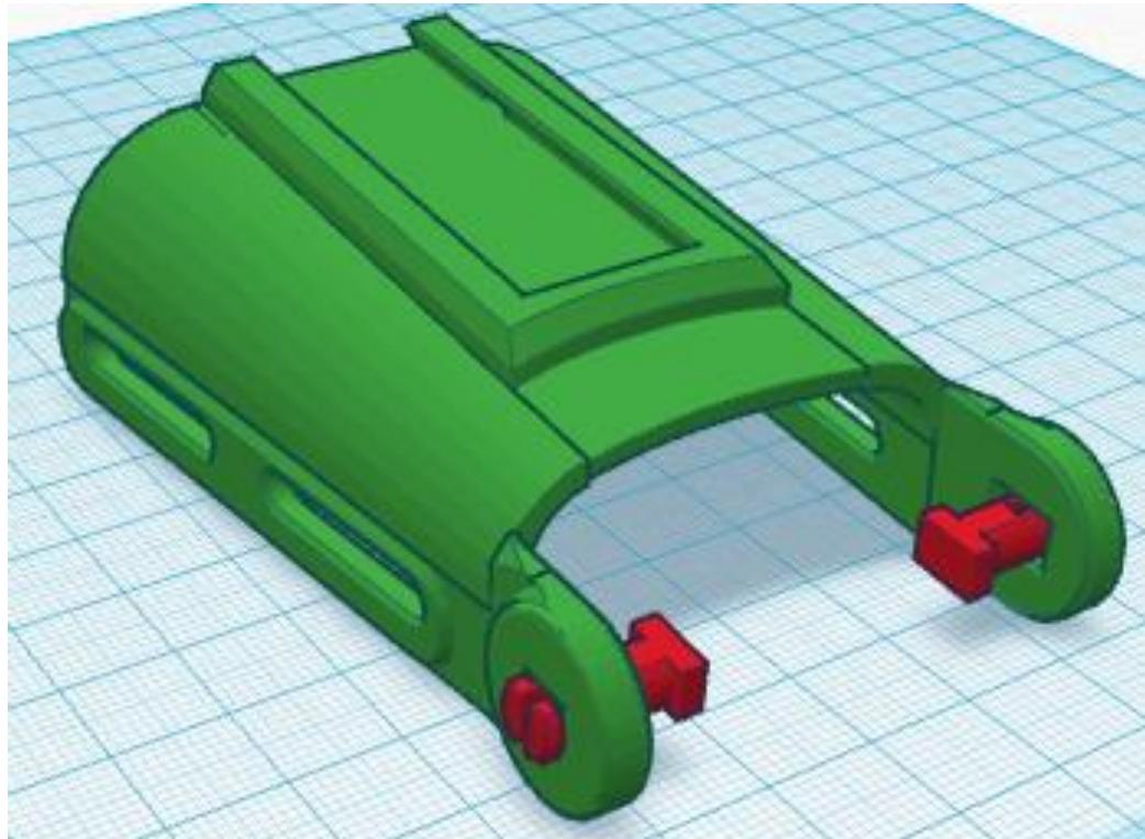
Press the wrist pins into the rectangular holes in the gauntlet hinge. The pins need only protrude a short distance ... don't push them all the way in.
