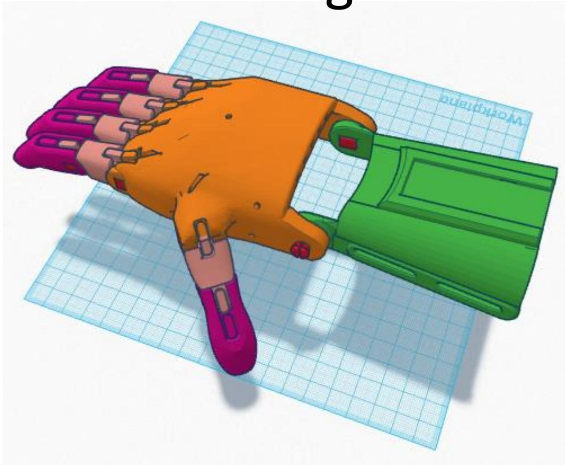
Slightly squeeze the gauntlet hinges together and locate the wrist pins in the corresponding holes in the palm. Press the wrist pins into place. You may need to use the pliers for this step.
