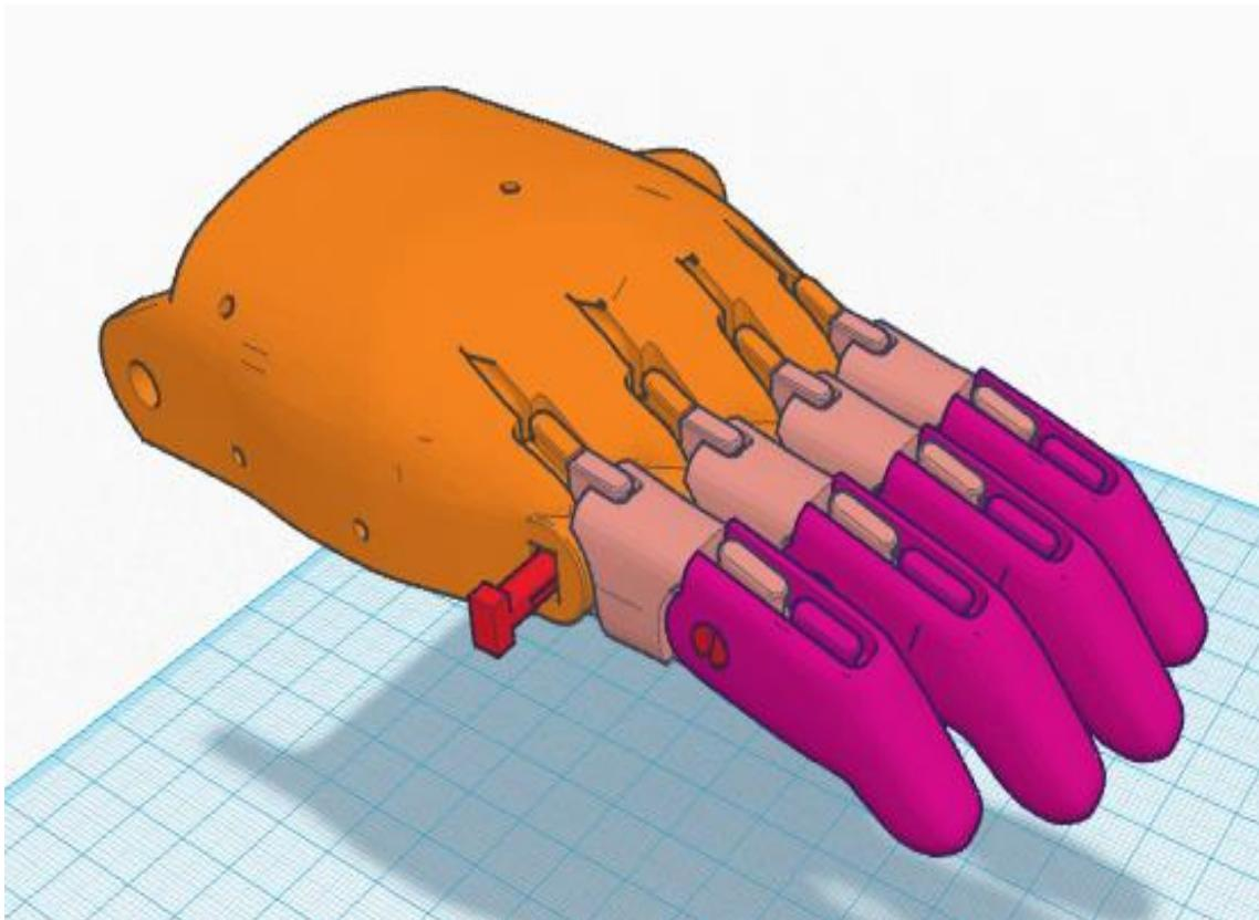
Before inserting the other short knuckle pin ensure that its rectangular head will fit in the rectangular pinkie finger hole in the palm. If necessary file or sand the pin head to fit.
