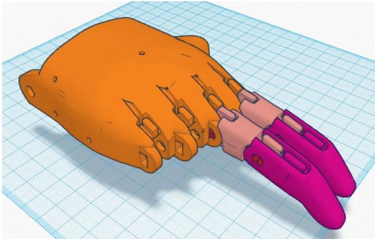
Insert middle finger into its joint slot and press the long knuckle pin in completely using the pliers. You may need to use a few light taps from a hammer to finish pushing in the pin but be very careful not to damage the outside palm joint for the pinkie.
