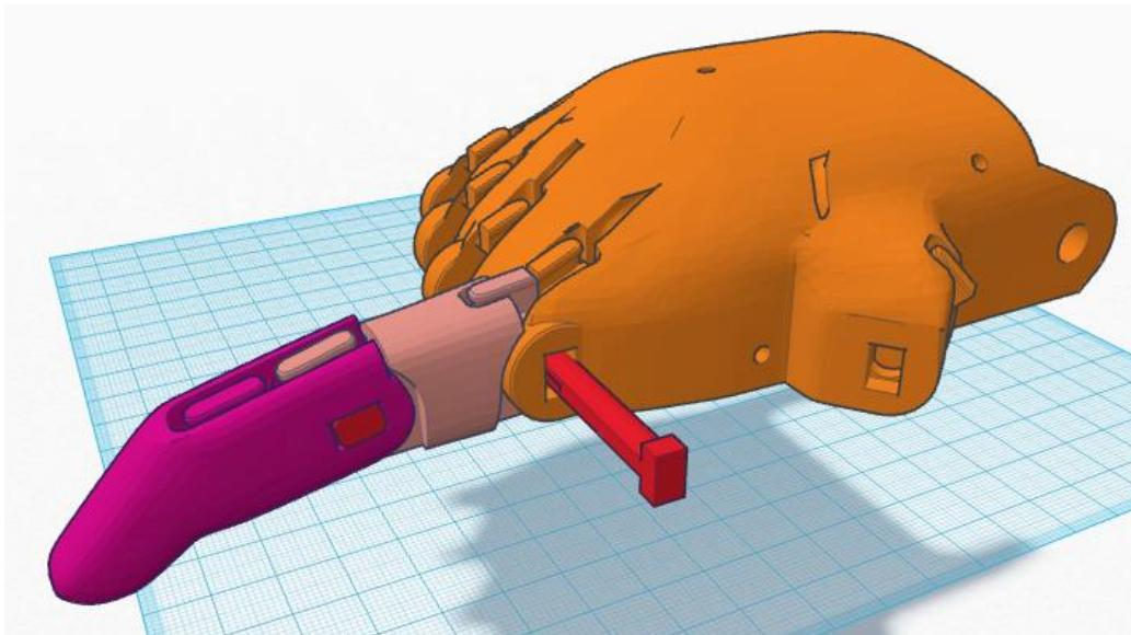
If you can't insert the pin try filing a 45° chamfer on the tip of the pin then try again.
