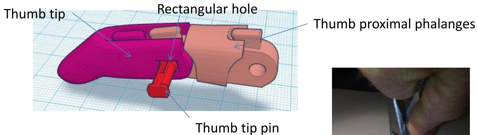
With the rectangular hole on the top align the holes in the thumb tip and thumb proximal phalanges (the wide one).
