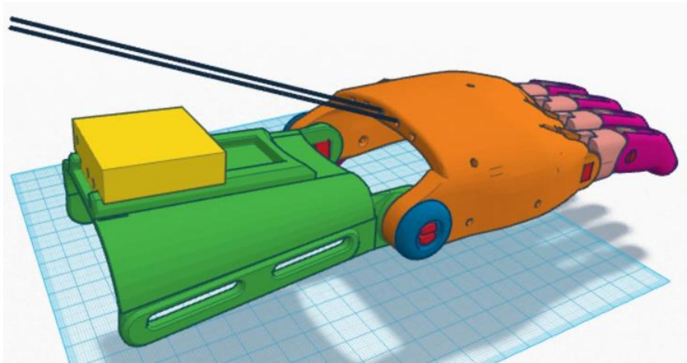
Cut another similar length of thread and repeat the operation using the middle hole in the back of the palm. Tie a knot on the bar under the middle finger.
