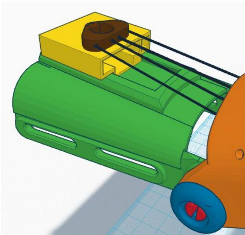
Repeat the stringing procedure but this time passing the thread from the middle finger through hole 2 in the whippetree and back out of hole 1. Then thread it through the second hole from the thumb side on the back of the palm down to the index fingertip but don't tie it to the bar on the fingertip yet!
